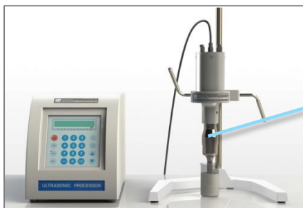
Figure 1a. LSP-500 in batch mode using a conventional horn (CH).
